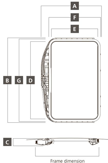
\*To provide for optimal positioning, the NSG can be delivered with the motor in the front or rear part of the frame component. The dimensions of the spoiler roof are identical in both versions.
